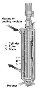
Fig. 2.8 Scraped surface heat exchanger for processing medium and high viscosity liquids, including those with particulates. (Courtesy of Tetra Pak.)
